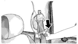
**Pulling Out Belt and Latchplate** 2. The seat belt latch plate is above the back of the front
